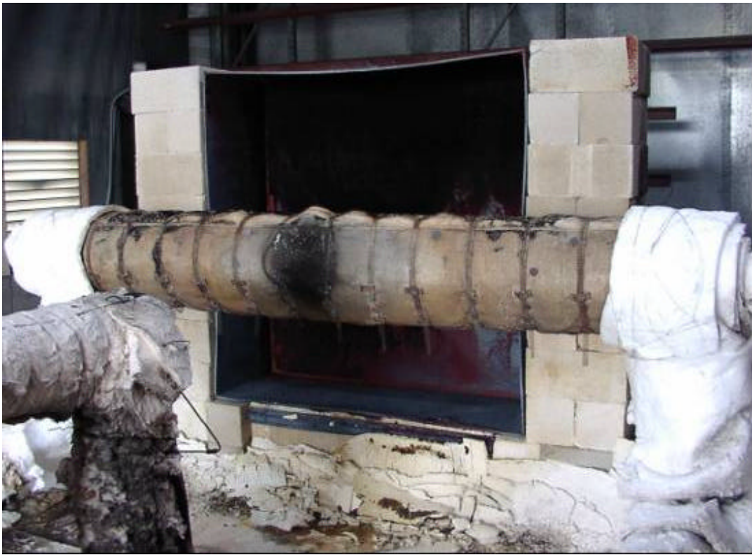
Figure C-5. Jet-Fire Test Specimen Immediately After Test.
