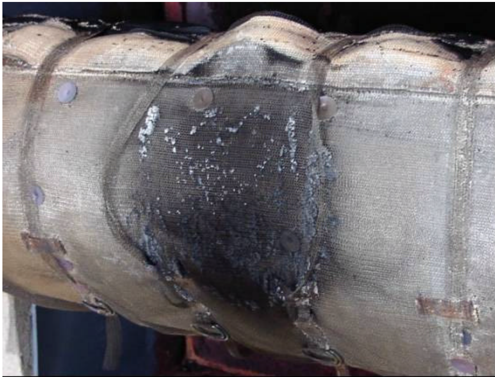
Figure C-6. Jet-Fire Test Specimen Impingement Region after Cool-Down.
