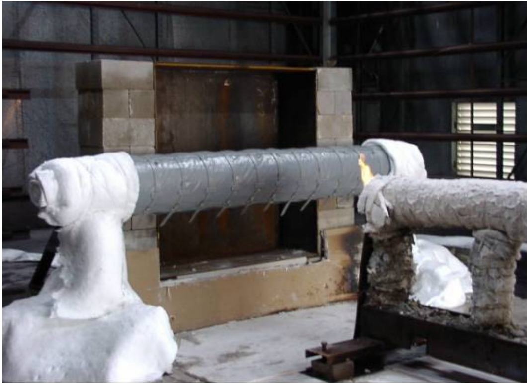
Figure C-2. Jet-Fire Test Jacket Assembly Prior to Exposure.
